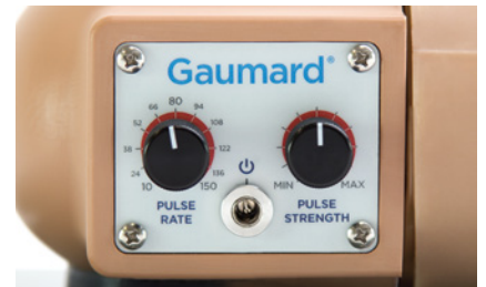
Micropump-controlled arterial system provides variable pulse rate and pulse strength
